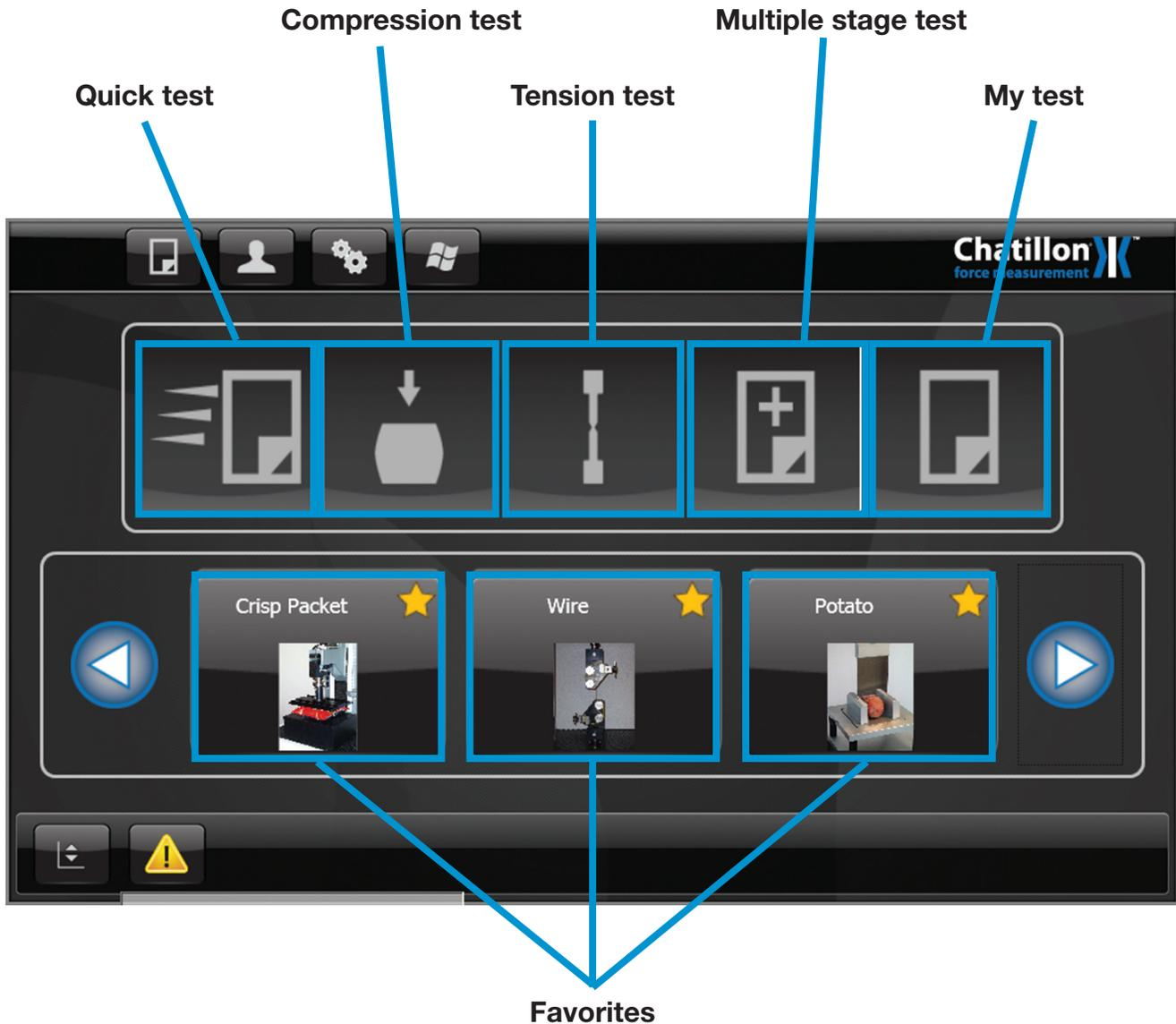
The CS Series has a 8.9" industrial-grade touch screen (IP65) that has been designed for easy continuous operation in a production environment. The screen is dust protected and can withstand liquid spills and splashes. The touch screen is not only rugged; it is also easy to operate, making it the perfect interface for users regardless of their skill level. A few touches are all it takes to set up a test, select test runs and present reports.
