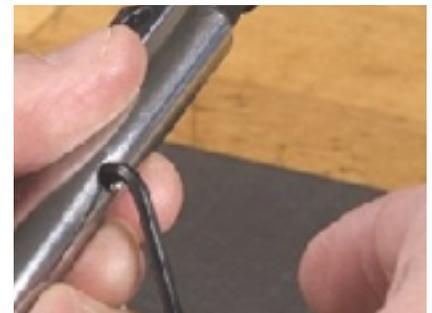
6. Rotate the grip and adjust torque to 20% of rated capacity. This is the lowest graduation +0 on increment.
