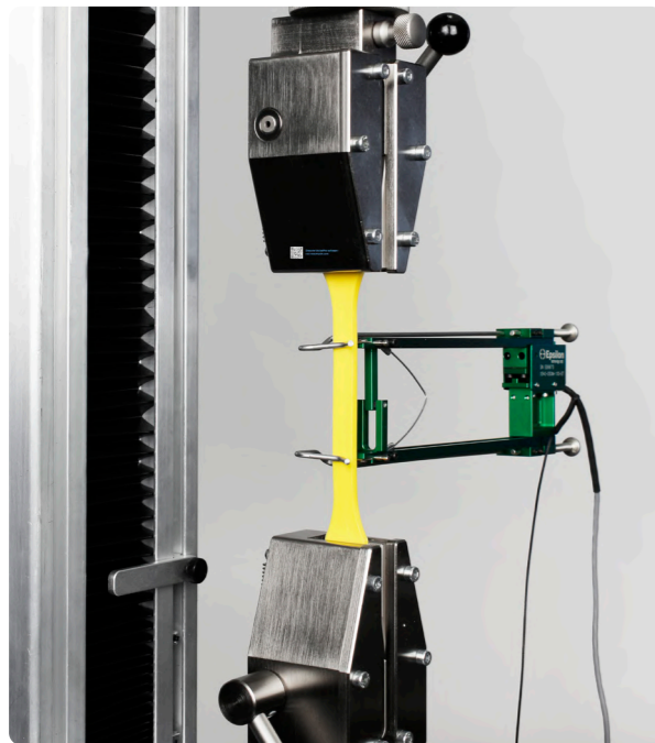
▲ Short-travel axial extensometer
